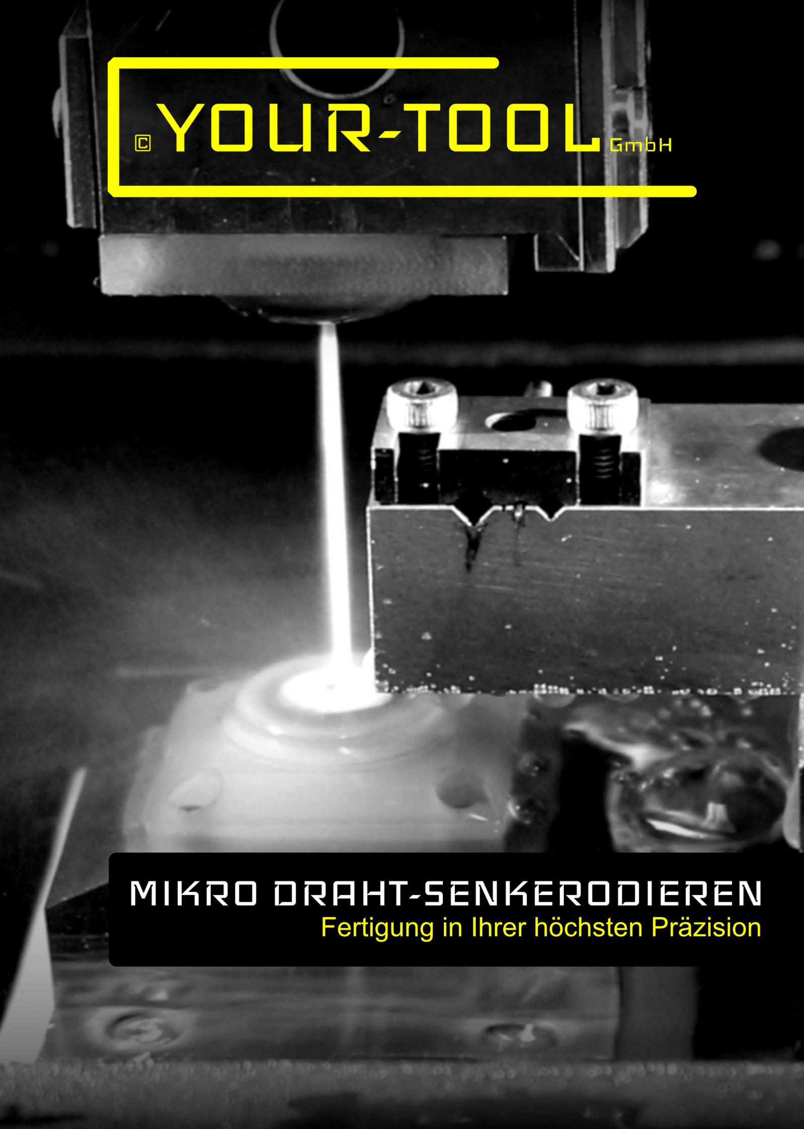
A black and white photograph showing a micro-wire EDM process. A thin wire is cutting through a metal workpiece. The wire is held in a fixture above the workpiece, and a small amount of metal is being removed. The background is dark, and the workpiece is illuminated. The text 'YOUR-TOOL GmbH' is overlaid in yellow at the top.
